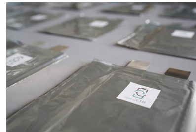
RecyLIB battery cells – alternative processing for direct reuse of recycled battery materials © Fraunhofer ISC
